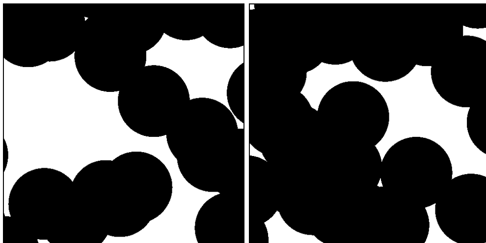
Figure 4.5: Two independent realizations of a Boolean model with discs of constant radius and parameters R = 0.15 and \lambda = 20
