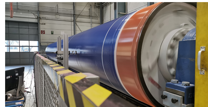
Above: Full-surface inspection of press sleeves for internal defects. The automatic AI-based evaluation takes place in the background.
