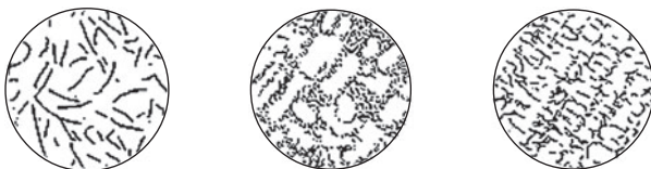
Standard series images for A-, D- and E-graphite.
