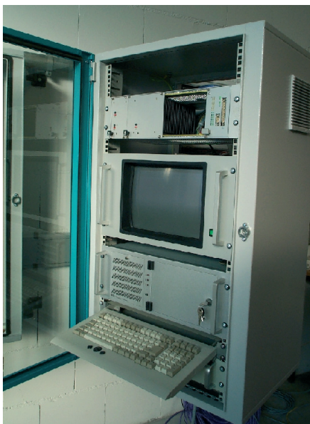
Evaluation electronics: the data measured at the sleeper are processed by evaluation computers with an infrared interface located at the tracks, and transferred to central systems. Large numbers of systems of this type work in several European countries.
