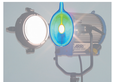
Temperature field simulation: in a floodlight, heat is mainly concentrating in the upper section.
