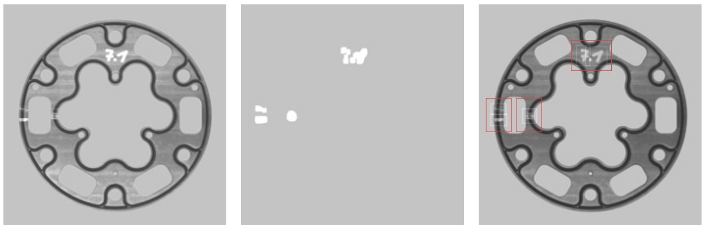
Surface inspection of a gasket (from left to right): original image, defect areas, marked defects
