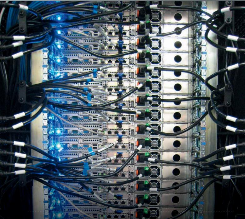
Back side of the computer racks: Separate data arrays are stacked in such "cabinets" and connected to each other in fast networks, for example, Infiniband. The close packing and linking of several such racks creates a mainframe computer that provides modern data centers with the computing power required for future-oriented HPC applications – like Deep Learning or other types of simulation.
