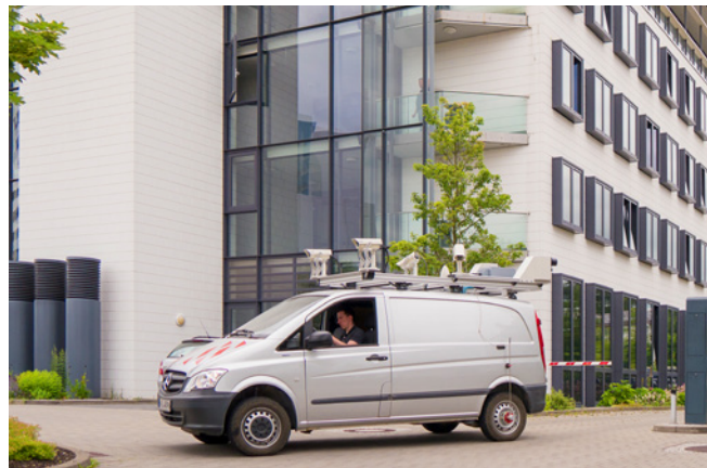
On the move with REDAR: 360-degree laser scanners detect the environment with high accuracy.
