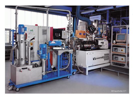
Fraunhofer ICT has a modern pilot plant with twin-screw extruders from 16 to 43 mm as well as versatile metering options at its disposal.
