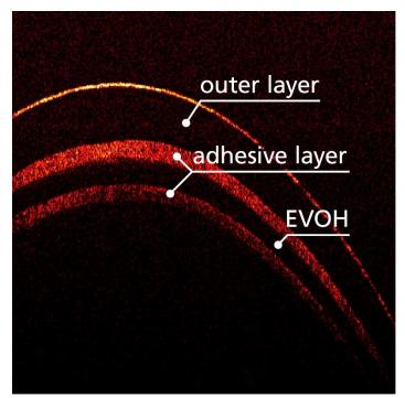
Labeled microscope image of a plastic tube. © Fraunhofer ITWM
