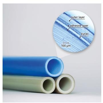
A multilayer plastic pipe consisting of outer and inner layers with an EVOH layer bonded via adhesion promoters in between. © Fraunhofer ITWM
