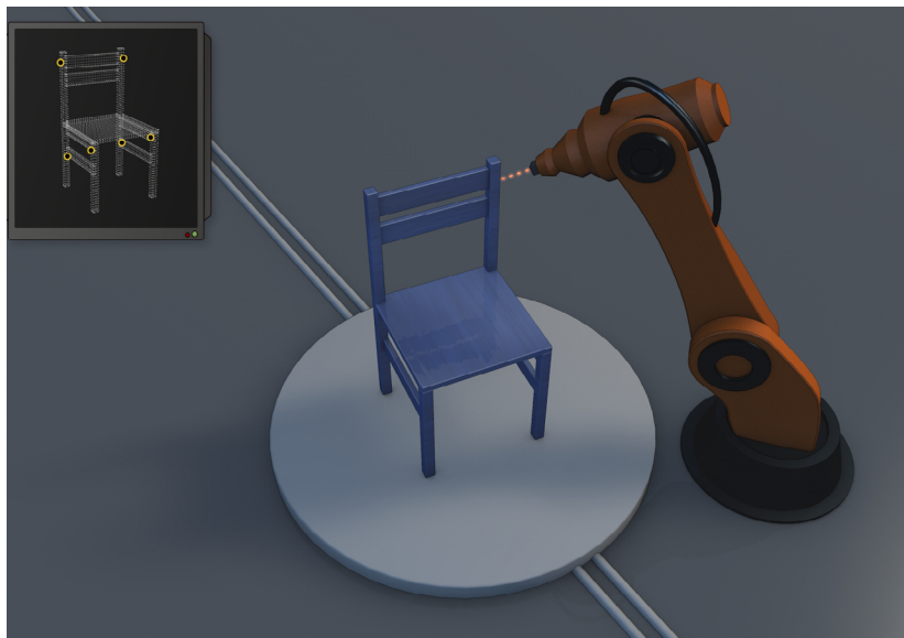
Schematic representation of the measurement process, in this example for a chair.
