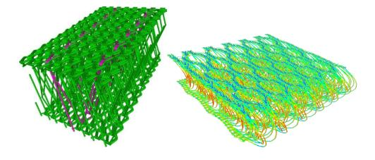
Visualization with marking of individual yarns, simulation of pull in the plane and further compression with software. TexMath. ©Fraunhofer ITWM
